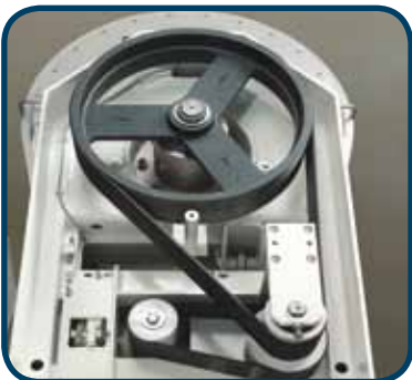
Mechanical reduction with pulleys and belts
