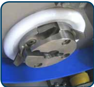
Mixing tool quick release system
