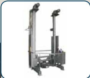
Bowl lifting and lowering with chains
